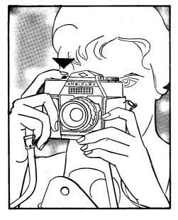
avoid blurring. Otherwise the camera should be placed on a rigid support or preferably screwed to a tripod.
