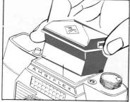
Open and close the waistlevel hood viewfinder by the knob on the lid. If the image is not visible in the viewfinder operate the rapid transport lever.
