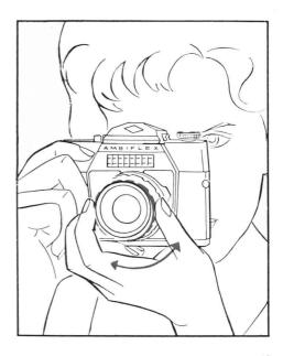
ing ring. You may also hold the camera with the right hand, supporting it on the palm of the left hand, and turn the focusing ring with thumb and index finger of the left hand, as shown in the illustration on page 23.
