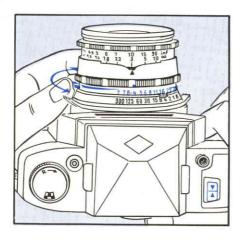
Turn aperture ring until exposure meter pointer is centred on the setting mark.
